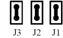
(d) J1, J2, J3 short circuit CW/CCW mode and active at high level (The fixed level)
