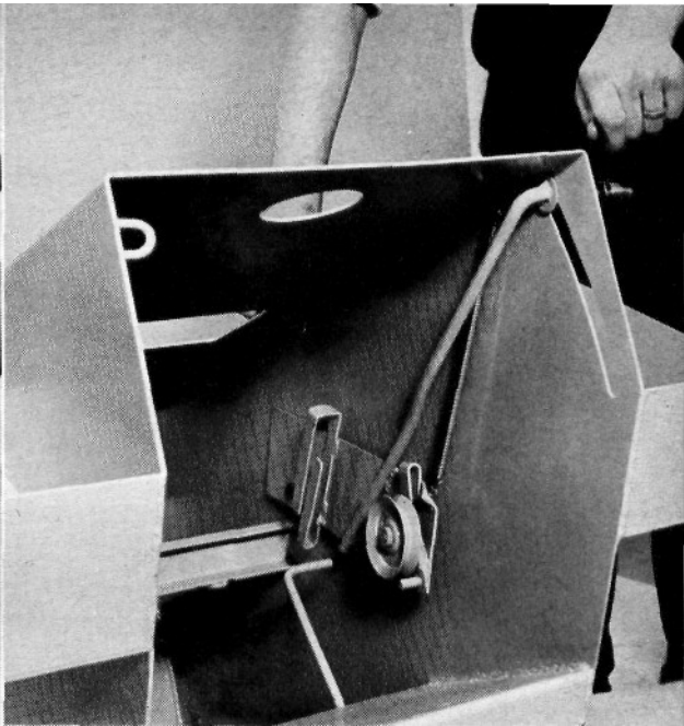
Reversing mechanism comes preassembled; you just bolt it to the tractor body. Left foot operates it.
