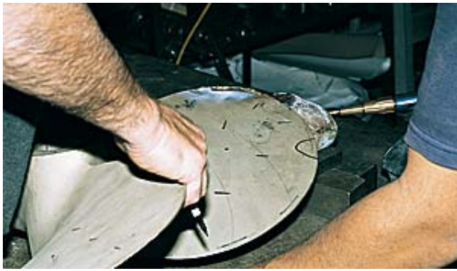
Damage or corrosion to propeller blades can sometimes be repaired, but it requires the skill of an expert. Do not try to do this yourself
